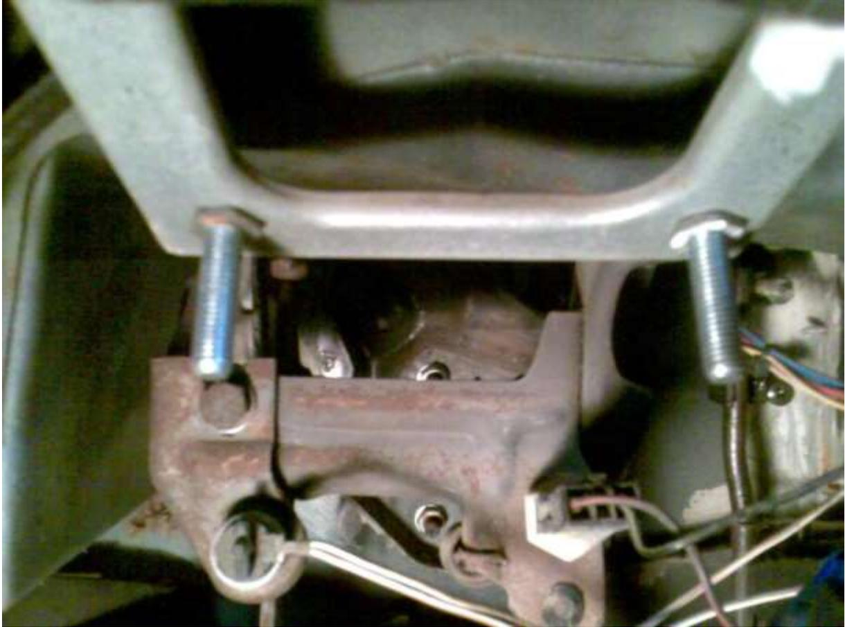
I used shallow nuts to hold the bolts in place as the bracket needs to be fairly close to the panel for alignment purposes. This should have the column in place now. You then need to cut the bottom off the Manta steering column like so...
