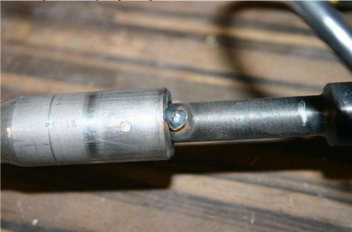
Upper mounts welded and new lower mount piece welded on
