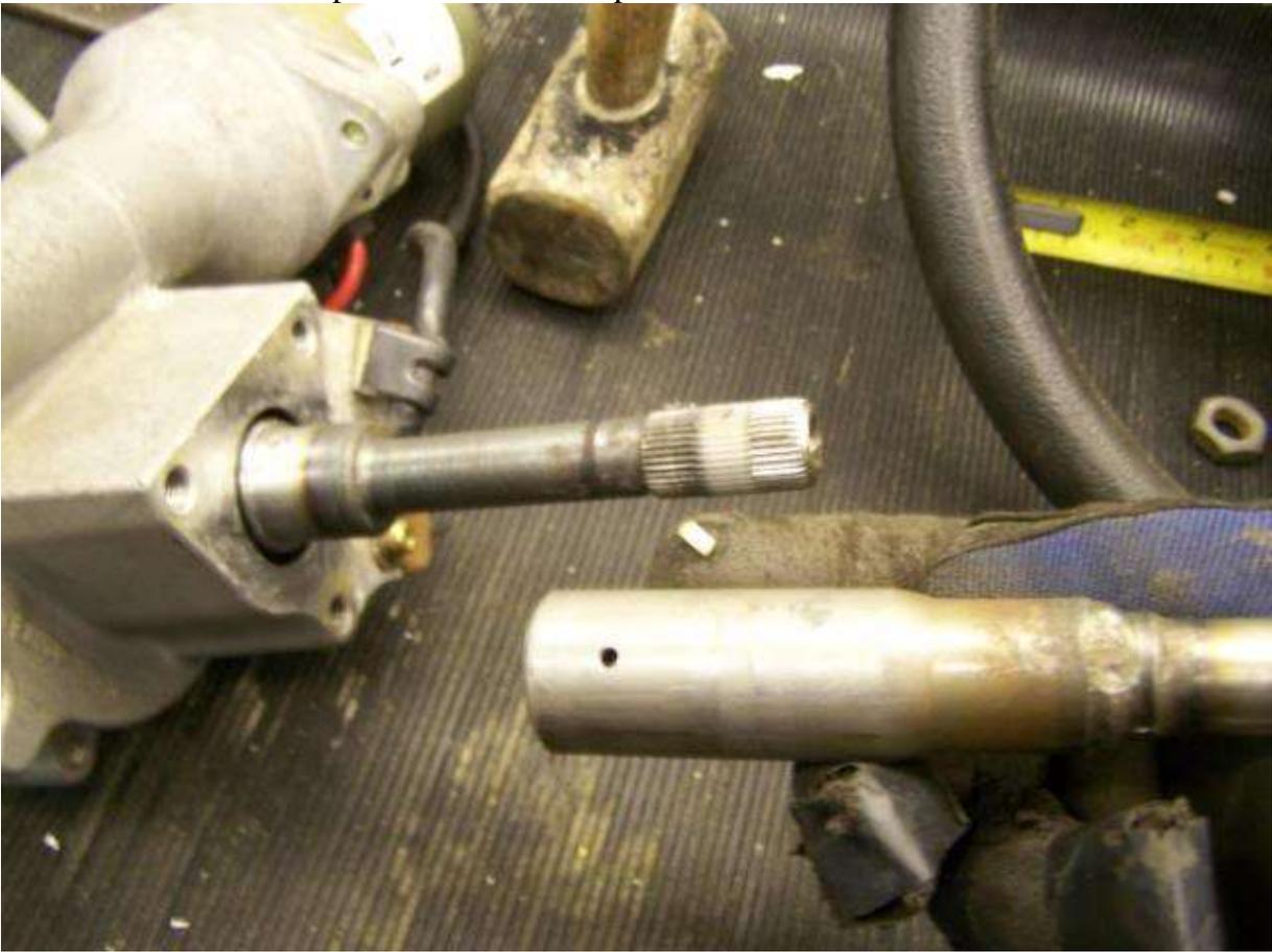
will be putting a blob of weld on mine to hold the 2 parts together as the top part with the manta bit added will not collapse now anyway, the reference for the amount to stick out is 85mm for the top part
