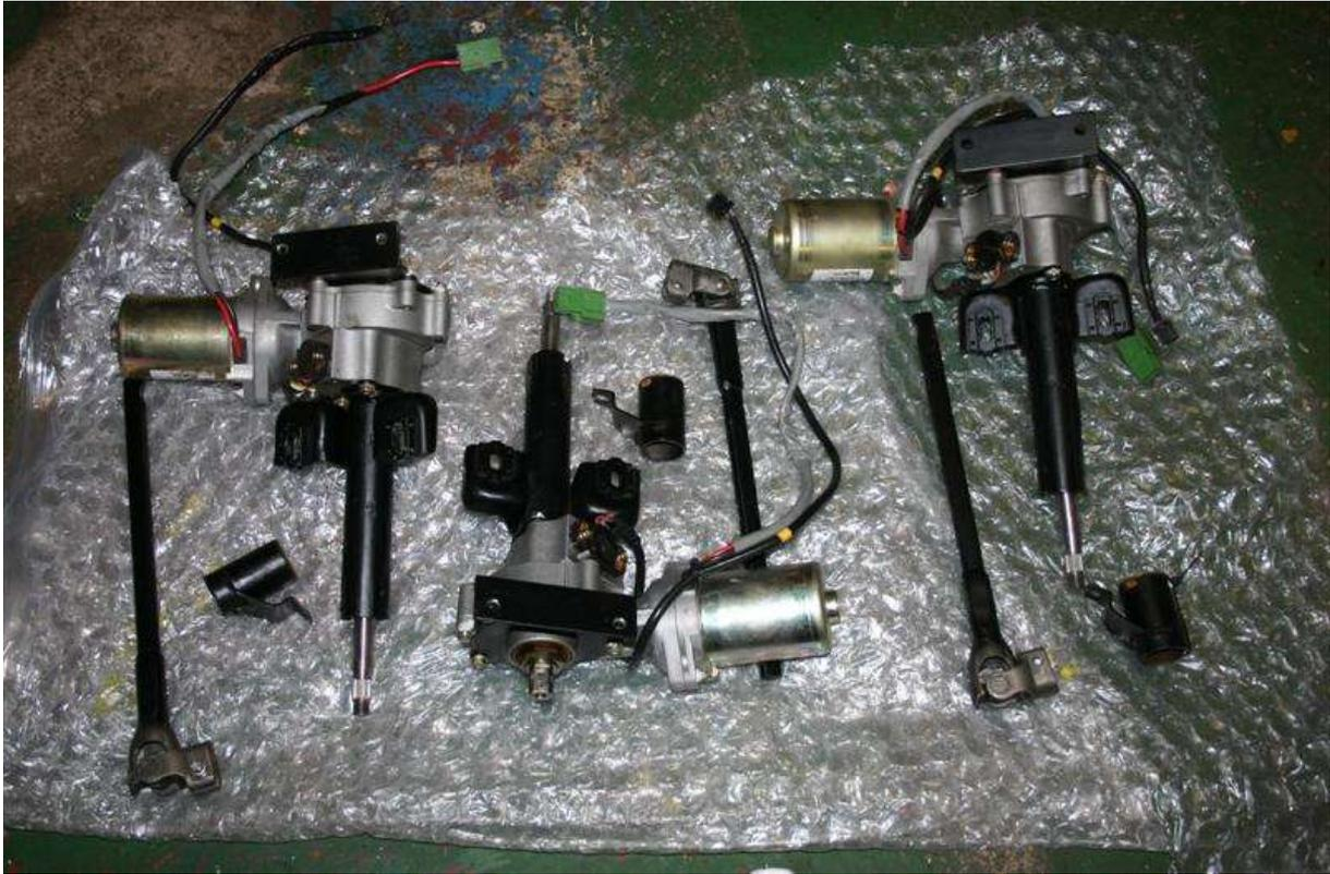
With this kit you get a modified corsa/manta column ready to fit to your car including a speed controller (required to make the column work).
