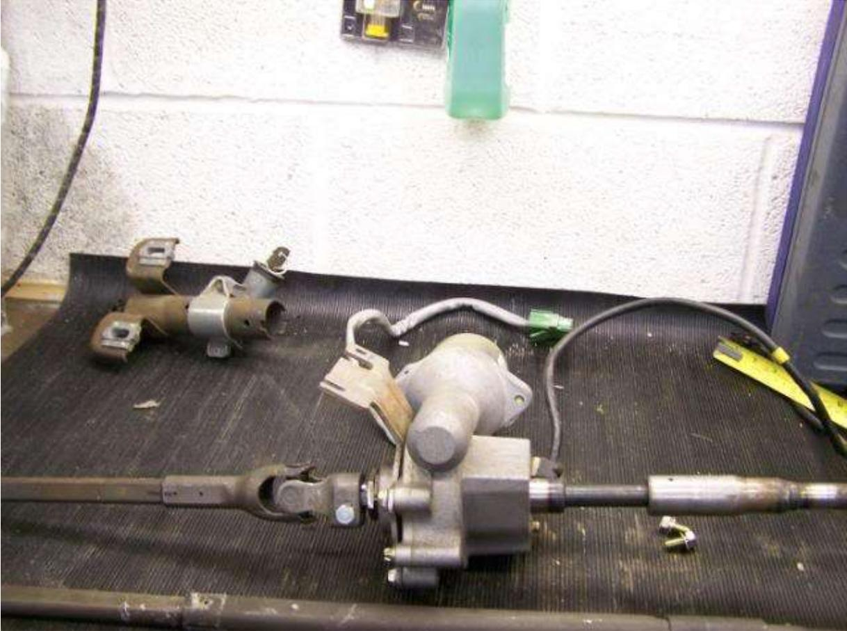
Take the bottom part of the outer of the manta column and bolt it to the floor, mine hasn't got a bearing in as it will be blasted and a new one fitted
