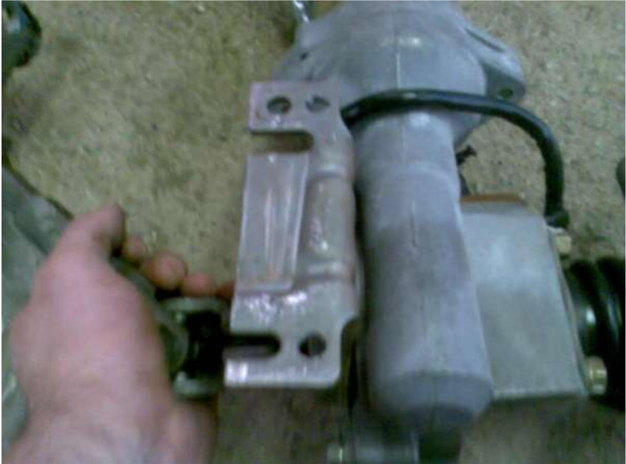
I then fitted 2 bolts to the Manta panel to mount the bracket to.
