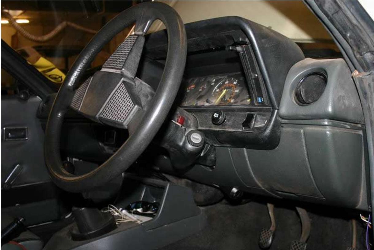
The mounting brackets have been made so the column motor tucks up behind the dashboard towards the passenger side so there is no need for major work to fit it. All that required is the drivers lower dash needs a small piece trimming out and the passenger lower dash needs a reinforcing web trimming back from the rear of it. You can just see the lower part of the column sticking bellow the dash, but this is not visable when driving or when stood next to the car looking in.
