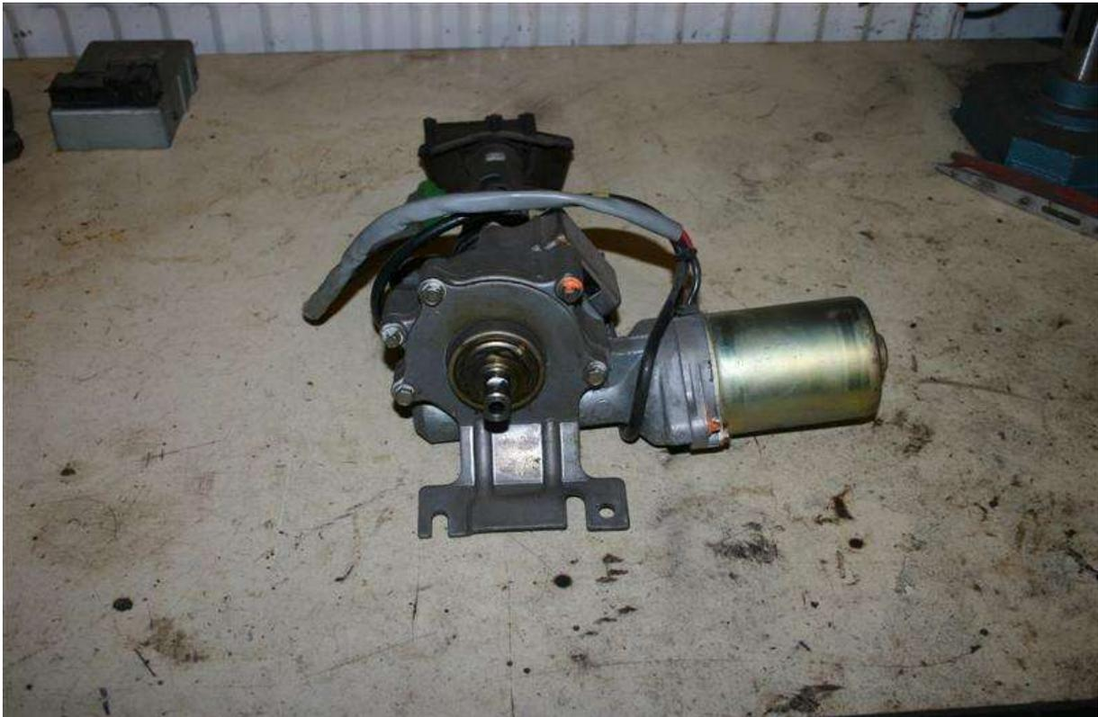
Then remove the lower bracket 3 x 10mm bolts
