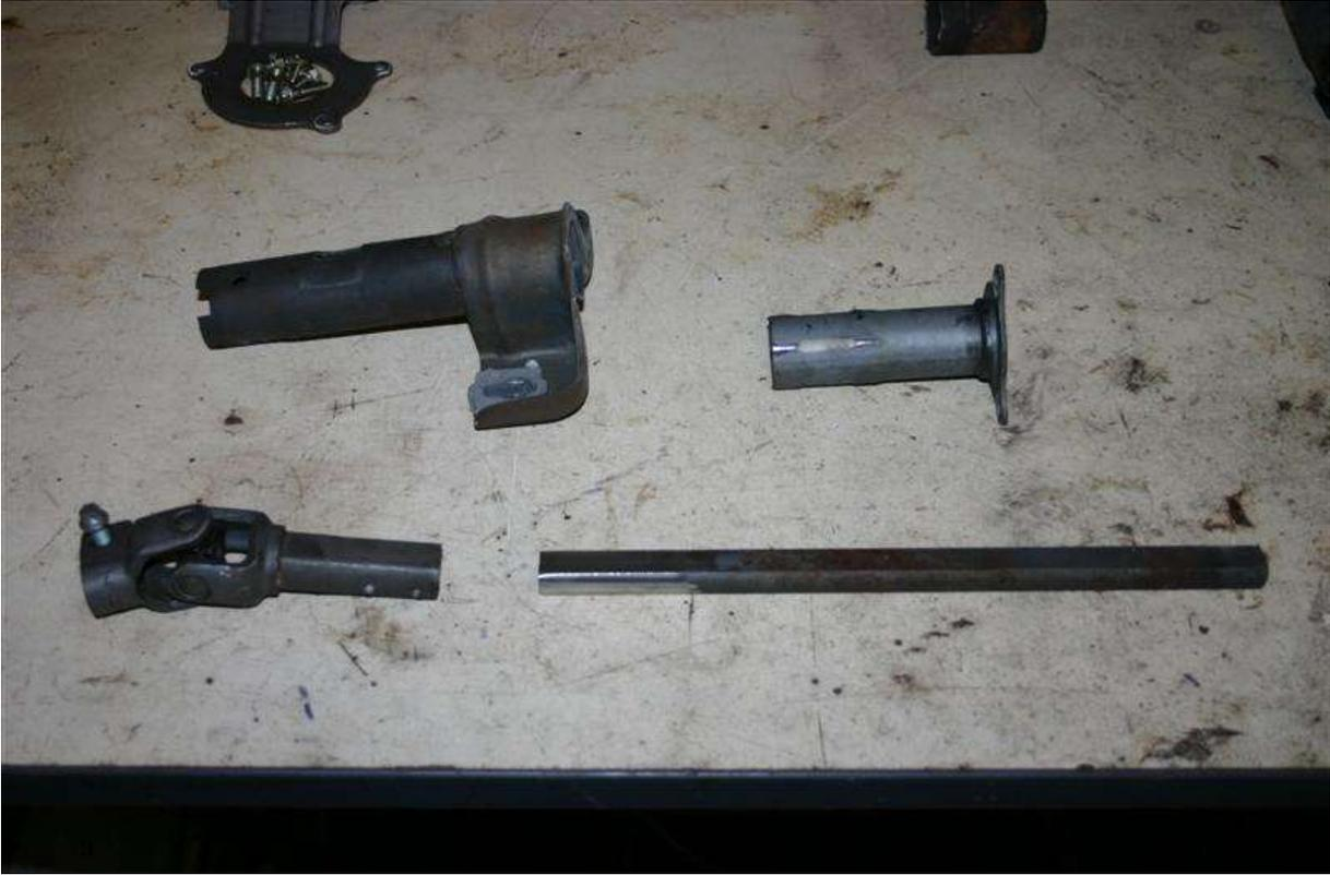
The corsa link u/j wants cleaning up and the holes drilling out to weld later
