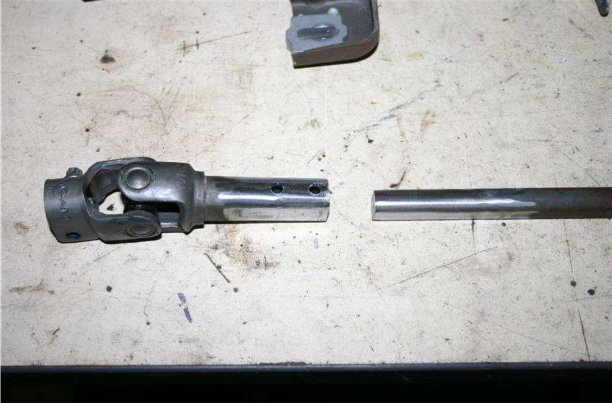
The corsa top shaft has a rough weld
