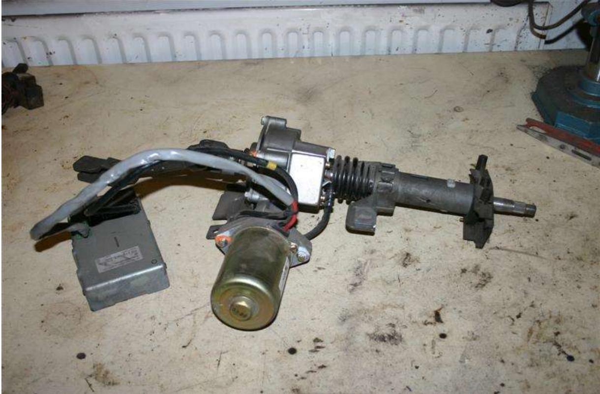
Remove the ecu and lower link
