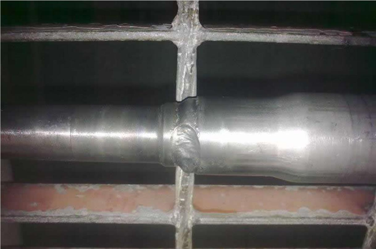
that needs smoothing to allow the manta bearing to fit
