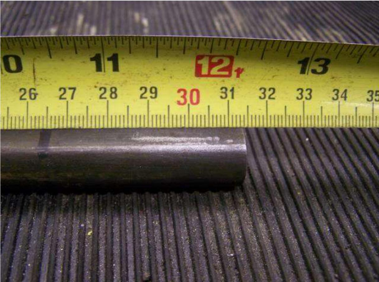
Shove that into the corsa UJ, it's a tight fit but this part if you leave unwelded will collapse in a front ender
