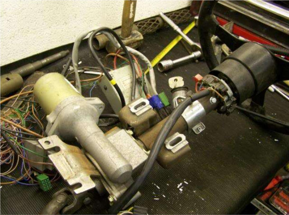
Bottom part of the column Take the inner shaft from the manta and split it then cut the bottom part down to 315mm
