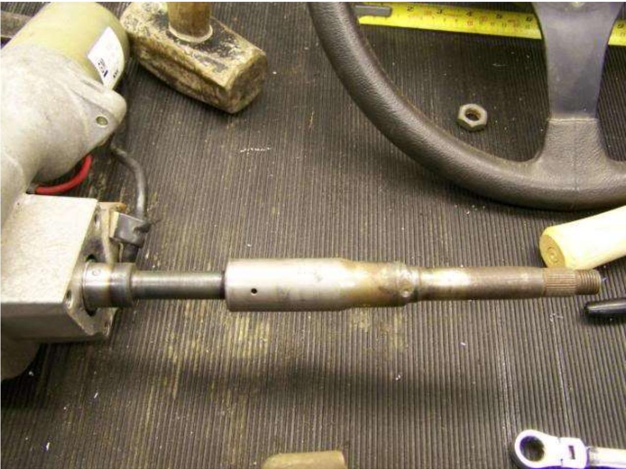
Don't hit the end of the spline as I did or the spline end will come off
