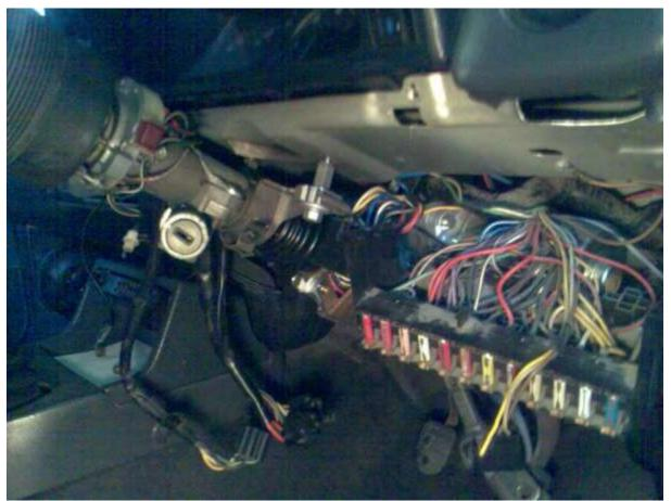
The bottom piece of the dash will need to be cut to allow the gearbox part of the Corsa column fit through but it can't really be seen. The fuse box will also have to be repositioned slightly. This takes time and plenty of patience. Hopefully this will be of some use to someone else on here. I'm sure I left loads of important stuff out but I'll remember when people start asking questions
