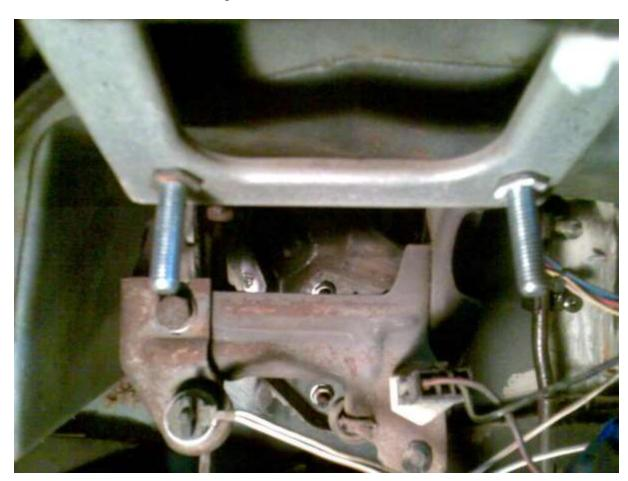
I used shallow nuts to hold the bolts in place as the bracket needs to be fairly close to the panel for allignment purposes. This should have the column in place now. You then need to
