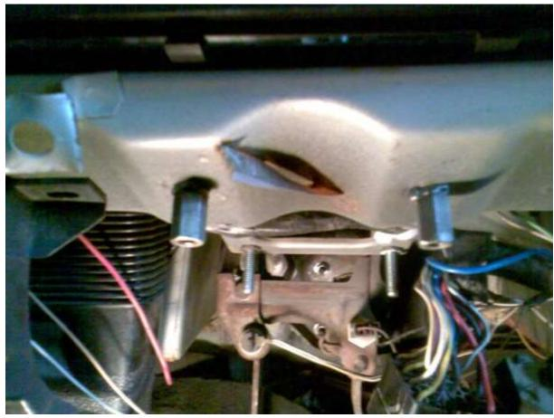
The rear of the Corsa column which houses the motor part of the column also needs to be fixed to the Manta. Thankfully Opel were kind enough to fit a panel above the steering column which is just right for the job. The bracket on the Corsa column needs to be bent like below and then 2 new holes drilled to line up with the Manta panel.
