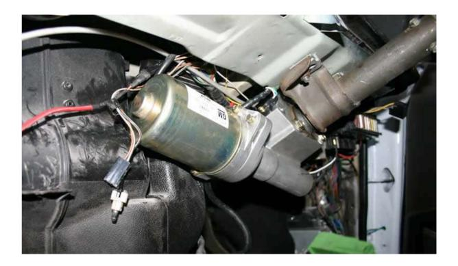
The lower dash needs a small amount cutting from the drivers side, and the passenger side needs a reinforcing web trimming down to make room for it. Other than that 2 holes need drilling for the extra rear mount on the column and 6 wires need connecting.
