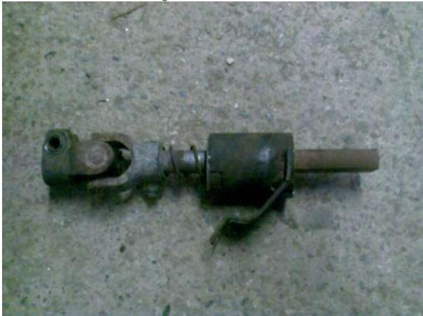
The piece that bolts to the bulk head needs to have a nylon spacer 40mm long inserted into it to keep the column straight in it. The cut end of the column fits into the Corsa column and the other end bolts to the Manta rack. There might need to be some adjustment made to get it all lining up right. I still need to adjust mine a bit but it works fine.
