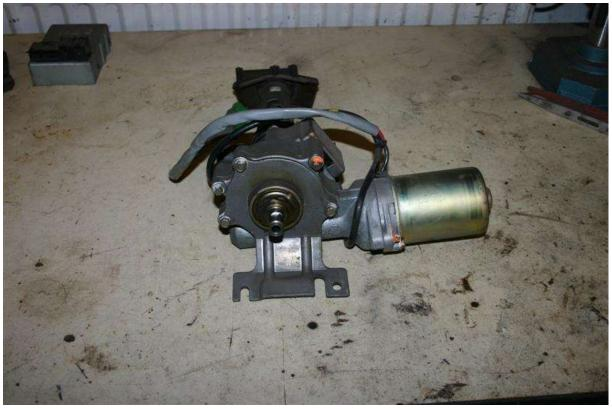
Then remove the lower bracket 3 x 10mm bolts
