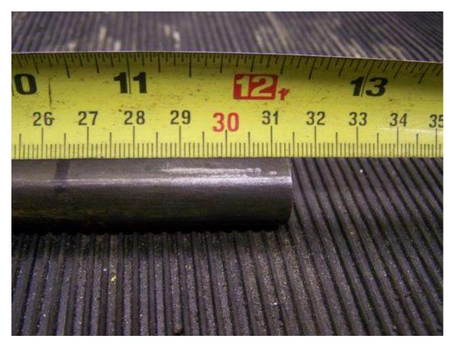
Shove that into the corsa UJ, it's a tight fit but this part if you leave unwelded will collapse in a front ender
