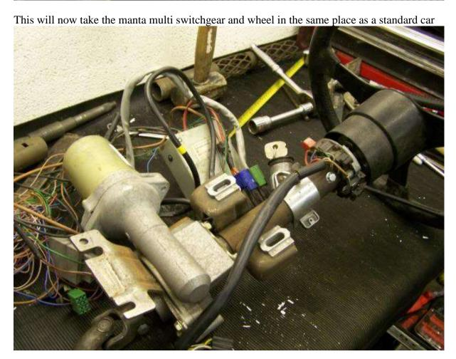
Bottom part of the column Take the inner shaft from the manta and split it then cut the bottom part down to 315mm
